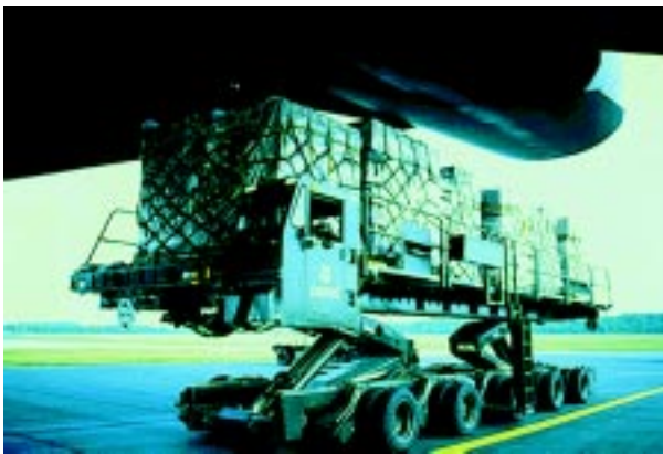
The Tunner 60,000-pound loader was the number two acquisition project in AMC. It could carry up to six cargo pallets at a time, loading and unloading cargo from military and commercial aircraft.
