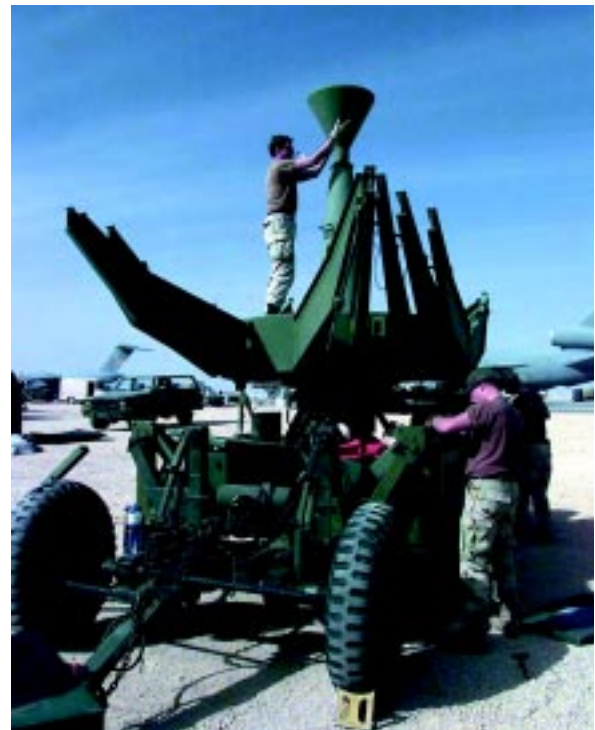
Installation of a quick reaction satellite antenna gave deployed forces in Southwest Asia direct communications with planners in the United States during Operation Phoenix Scorpion II.
