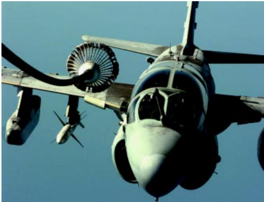
Configured for probe and drogue air refueling, a KC-10 Extender refueled a US Navy EA-6B Prowler over Southwest Asia during Operation Southern Watch. Because of the wide variety of aircraft with diverse refueling systems employed in Southwest Asia, the KC-10 was a coveted asset in the theater because it could be configured for boom as well as for probe and drogue refueling.
