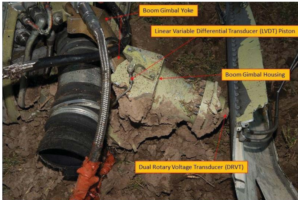
Figure 7 - Boom as found in field
