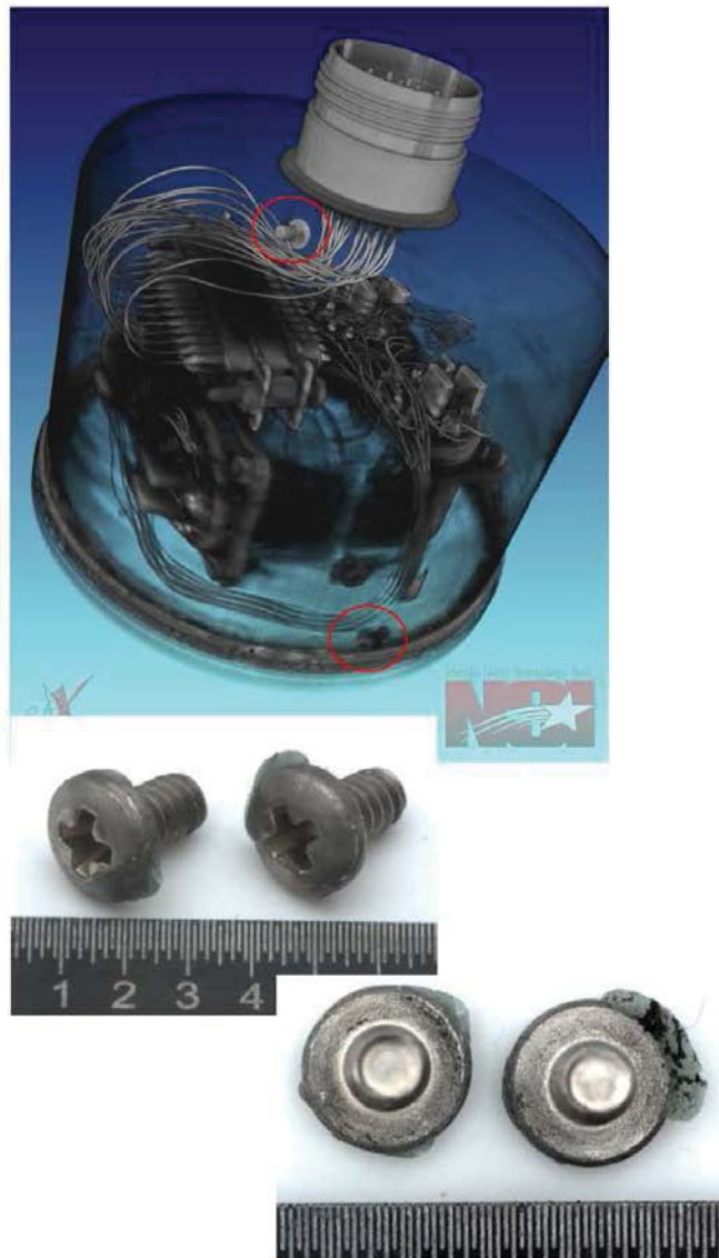
Figure 9. Examination using computed tomography revealed two loose screws within the sealed accelerometer. The screws were removed by milling a hole in the upper surface of the case. There was no evidence of arcing or thread stripping on the screws.
