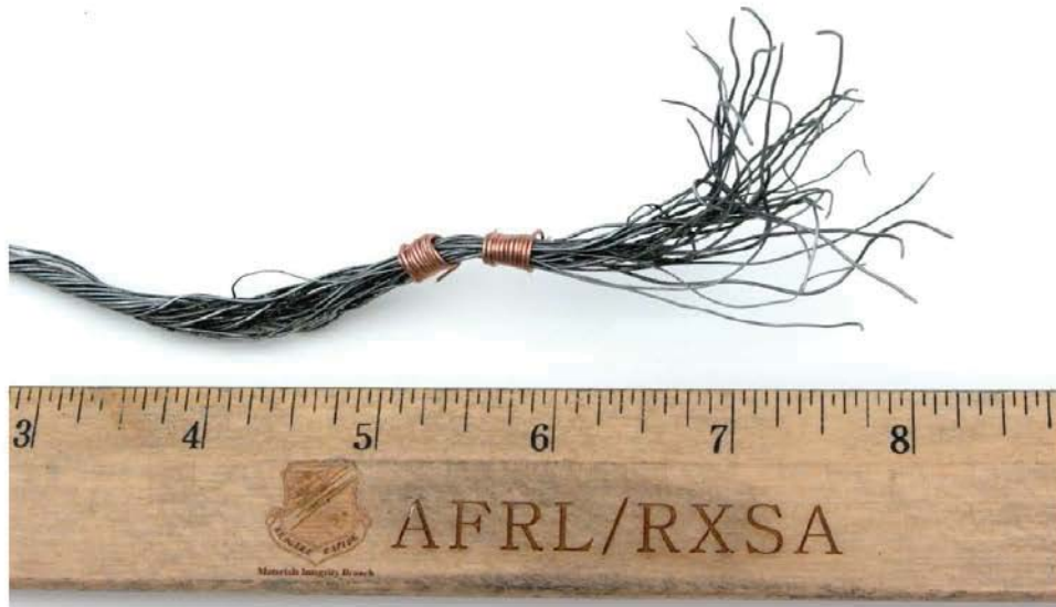
Figure 6. Copper wire was used to bind the wires within a strand together to preserve their relative position after sectioning.
