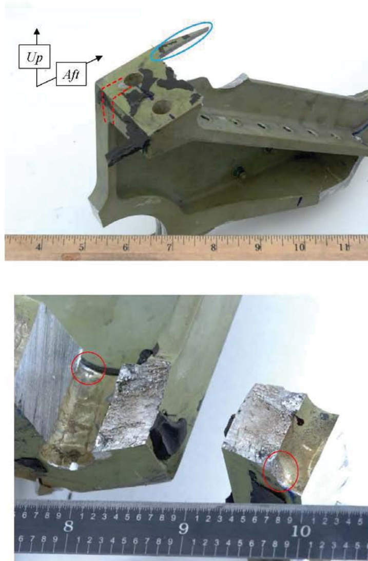
Figure 10. A through crack was noted at one bore (red dotted lines). The red ovals indicate coating distress was noted on opposing ends of the bore (red ovals), which indicates the fastener is loaded in bending. The blue oval indicates the location of the fracture surface shown in Figure 12 .
