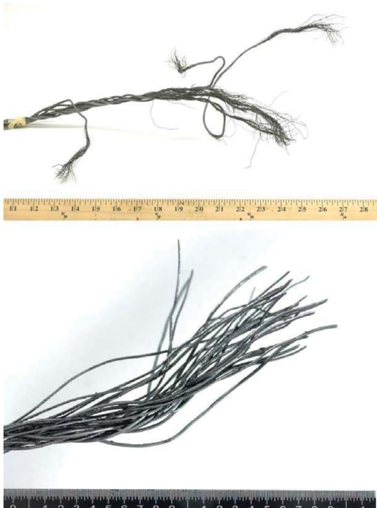
Figure 3. The fractures of each strand were somewhat displaced from one another (upper image), while the fractures within each strand were at approximately the same location (lower image).
