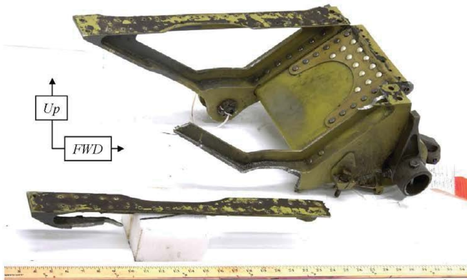
Figure 3. The submitted A-frame support, as-received. A portion of the fractured right-hand support was not submitted to AFRL.
