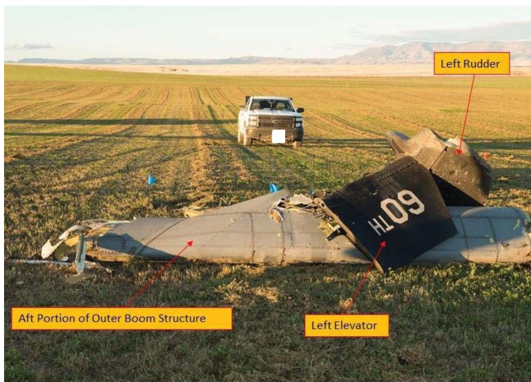
Figure 8 - Boom as found in field
