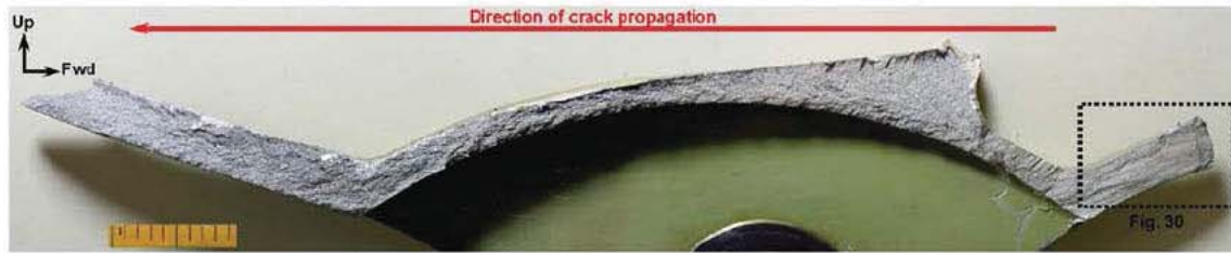
Close-up of fracture surface from L/H lug of Support Fitting clevis (Figure 6)
