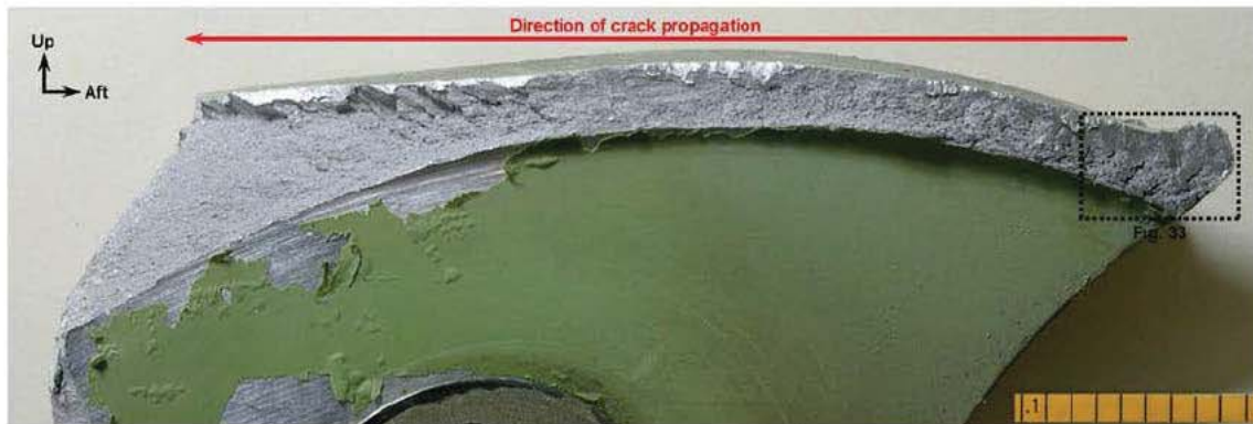
Close-up of fracture surface from R/H lug of Support Fitting clevis (Figure 7)
