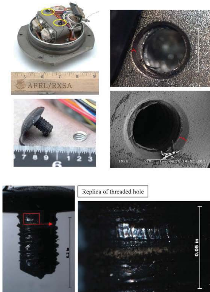
Figure 12. The threaded holes in the base plate were examined directly using stereo optical and electron microscopes, and by extracting Struers repliset black replicas. Curly brackets in the upper right-hand images indicate the chamfer. Sheared threads were observed directly, and smear marks consistent with axial stripping were noted on the replicas.
