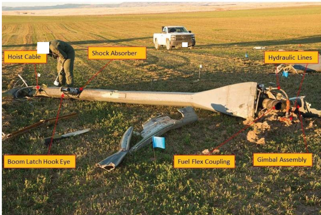
Figure 5 - Boom as found in field
