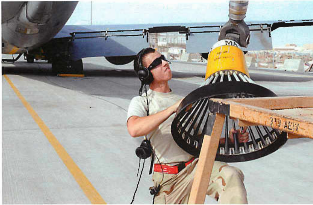
As part of the preflight checklist, Airman 1st Class Jason Somrak, serving with the 379th Expeditionary Aircraft Maintenance Squadron, muscles the KC-135 Stratotanker aircraft refueling pod off of the stand on the flightline of an undisclosed airfield in Southwest Asia, 10 September 2008. (US Air Force photo by TSgt Michael Boquette)
