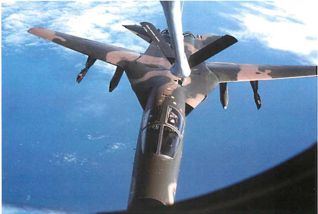
An F-111 aircraft is refueled by a 912th Air Refueling Squadron KC-135R Stratotanker during a refueling mission over the North Sea. (US Air Force photo by MSgt Patrick Nugent)
