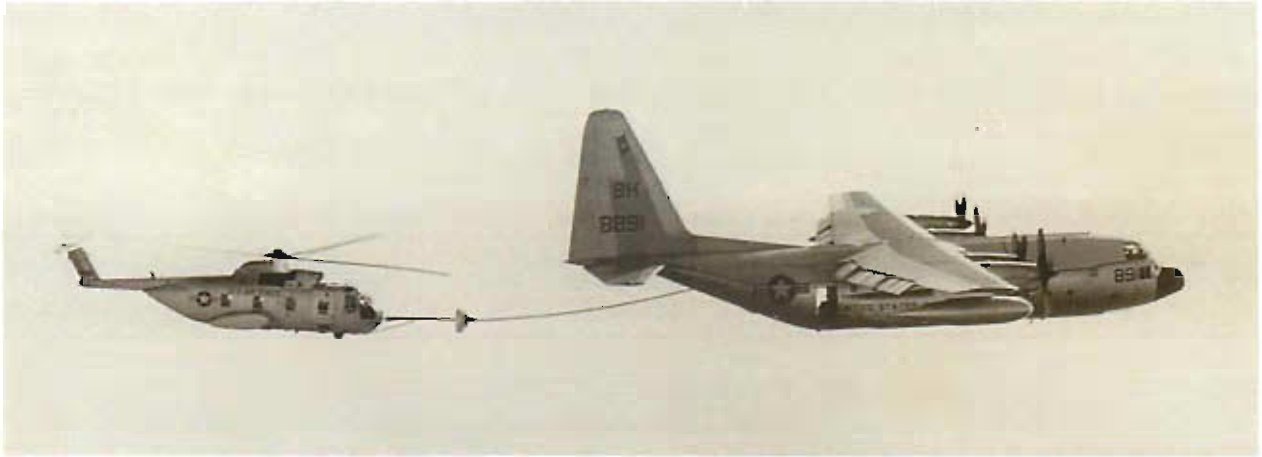
A CH-3, with a dummy probe, conducts an air refueling concept test with a KC-130 tanker.
